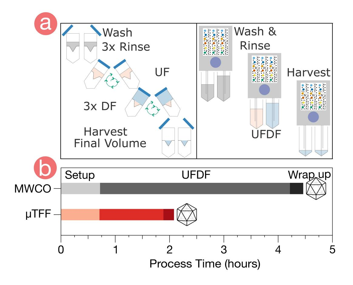
Figure 1: Comparison of the MWCO and μTFF Methods
